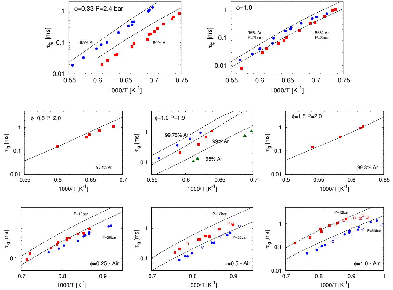
Ignition delay times fitted to indicated pressure (bottom - Ref. 3).
