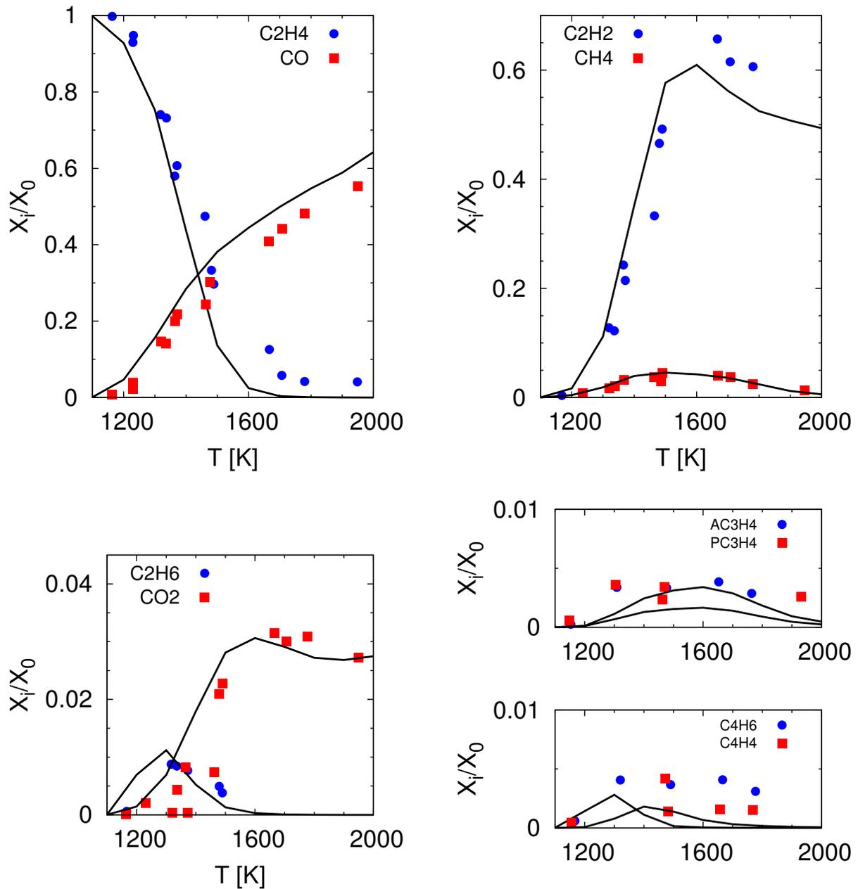
Species distribution during oxidation in a shock tube. Residence times and initial pressures as specified in Ref. Mixture D, 0.6% C<sub>2</sub>H<sub>4</sub>, 0.3 % O<sub>2</sub> in Ar.
