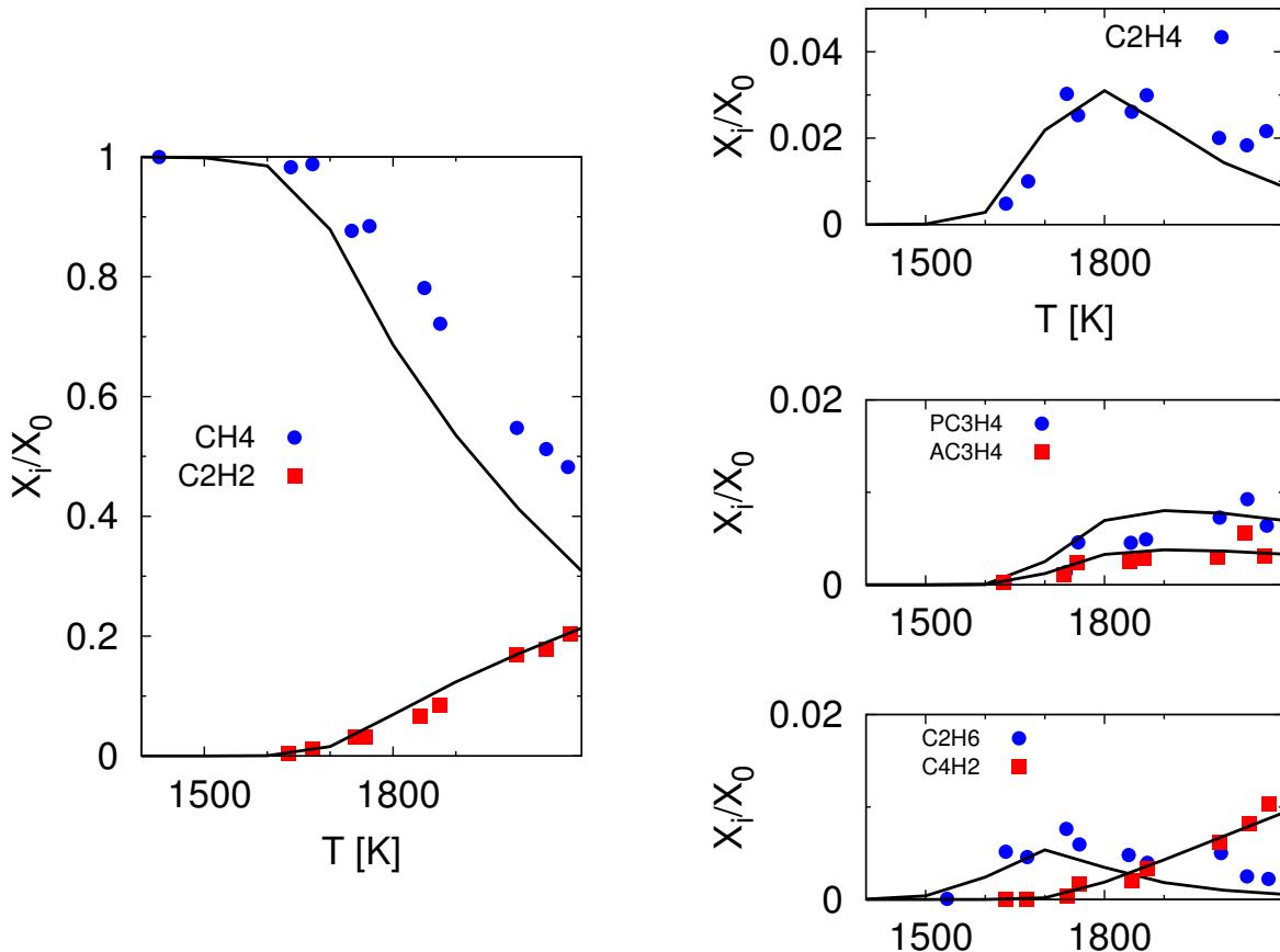
Species distribution during pyrolysis in a shock tube. Residence time and initial pressures as specified in Ref. Mixture A, 5% CH<sub>4</sub> in Ar.
