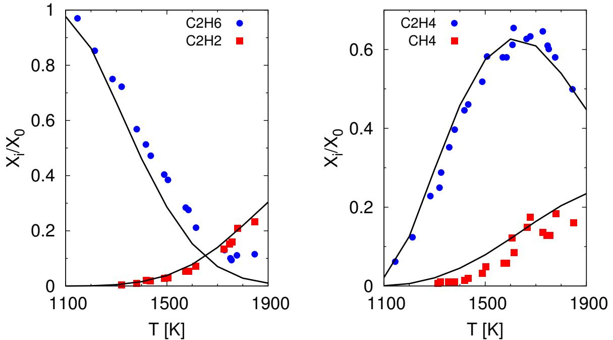
Species distribution during pyrolysis in a shock tube. Residence time and initial pressures as specified in Ref. Mixture A, 5% C<sub>2</sub>H<sub>6</sub> in Ar.
