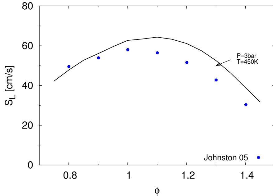
Outwardly propagating spherical flames (Johnston et al.).
